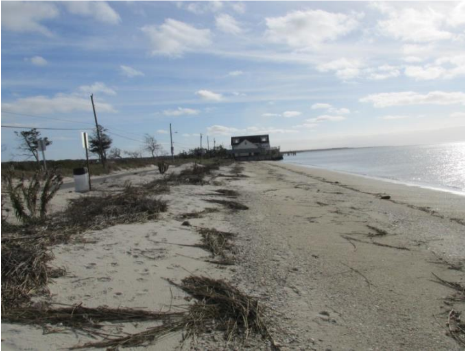
Figure 633a & 633b. The left photograph was taken on November 17, 2015. The right photo was taken on September 28, 2016. The left view shows the road and dune landward of the road and the new ridge of sand placed on the upper beach to hold back minor wave/storm events. The right view shows the beach slope to the low tide terrace with the recent swash line on the sand.
