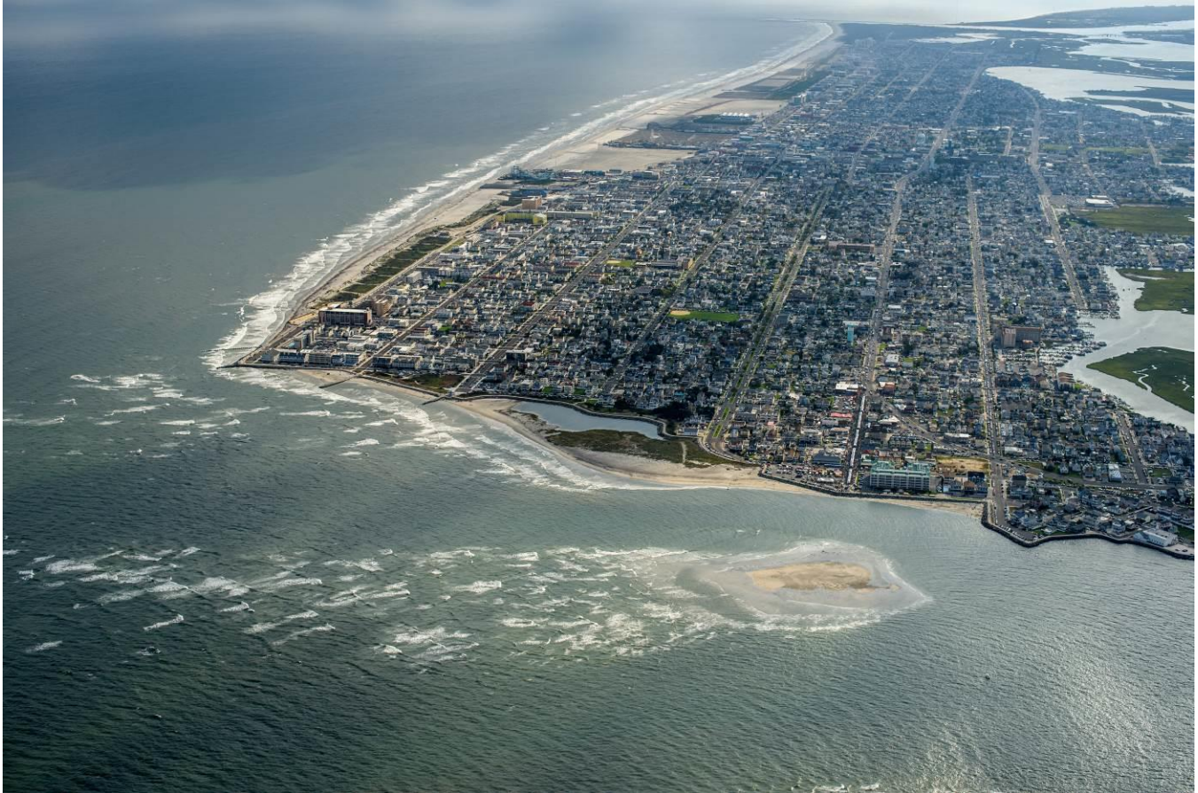
Figure 2. September 22, 2018 view from over Hereford Inlet looking southeast at the inlet shoreline, the new island shoal and the depleted oceanfront beaches. The island shoal was present in August 2016, but 350 feet further northwest up channel. The pattern of breaking waves indicate where shallow water exists presently and outlines the main tidal channel in the foreground northeast of the island shoal. The secondary channel lies between the shoal and the North Wildwood shoreline. To the northeast of the 2 nd and Kennedy Boulevard jetty there is a narrow, 8-foot deep channel which funnels sand into the inlet from the oceanfront beach, while immediately offshore from this channel there lies 50 acres of shoals less than 5 feet deep at high tide (November 2018 survey data). The inlet beach is eroding to the point where the Surf Avenue vehicle entrance ramp exits into the water, not on the beach sand and the small pond, present since the 1990's is again open to tidal flow across the beach every high tide. This island shoal needs to move two city blocks to the southeast and about 100 yards closer to North Wildwood to re-establish conditions at the inlet replicating those in place in 1995.
