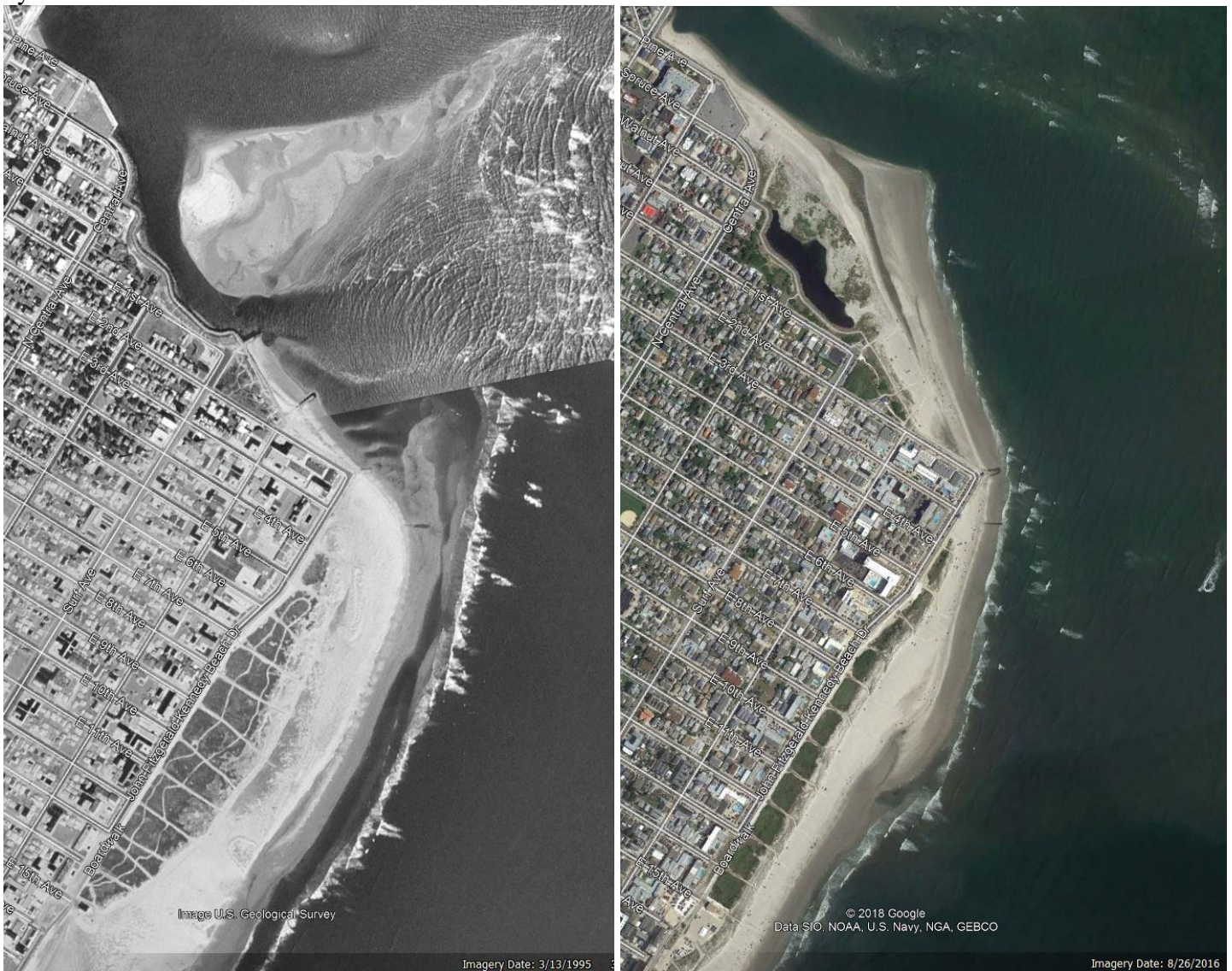
Figure 1. The northeast quadrant of the City of North Wildwood between March 1995 and August 2016 shows that oceanfront erosion appears related to large changes in shoal position and exposure at low tide in Hereford Inlet. In 1995, an exposed island sat between Central and Surf Avenues forcing a branch of the main tidal channel against the North Wildwood shoreline. There was no beach at the inlet shore until southeast of Surf Avenue. There was an extensive exposed sand flat system attached to the beach front bar system extending into the inlet. The ebb-tidal currents exited in proximity to the oceanfront beach and deposited sand in transport where wave action could easily move it to the beach bar system, and eventually onto the dry beach. In the mid-1990's the main channel shifted to the northeast, away from North Wildwood allowing the flood-tidal currents to move sand from the oceanfront beach into the inlet along the North Wildwood shoreline depositing the sand spit that has been present since. At its maximum extent (2001), this spit was over 600 feet in average width, with a pond created when the spit tip attached to the inlet shoreline near New Jersey Avenue (extended). As of the August 2016 view, the beach narrowed rapidly starting at 7 th Avenue to the inlet, but still showed a dry beach width at the inlet jetty. Sand was continuing to be transported into the inlet generating the new spit reaching almost to Central Avenue. Since then the main tidal channel has shifted more to the northeast and a new island shoal formed by 2011 with a secondary channel between it and the City's inlet shoreline. Since 2011, this shoal has migrated toward the inlet jetty further constricting the channel close to North Wildwood. This channel needs to close considerably before the 1995 conditions are re-established. Then and only then will the oceanfront beaches preferentially receive sand instead of shedding it both south into Wildwood City and northwest into Hereford Inlet.
