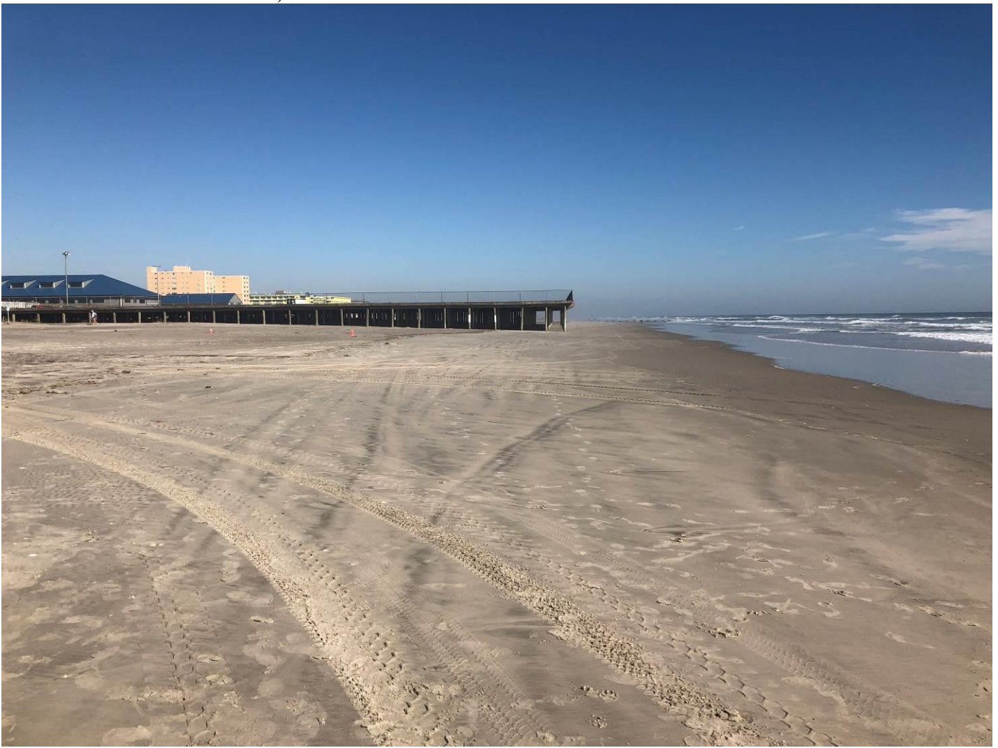
Figure 25. Site 60+00 was included this year in the survey plots presented, with calculations for sand volume and shoreline changes. The view was taken November 11, 2018. This site lies in proximity to 24 th Avenue, between the Surfside Pier and the timber pier to the north in the photograph. The dune lies well landward of the end of the pier due to post-2009 erosion. The as-built project dune extended seaward of all three piers and was exposed to wave erosion immediately by the 2009 Veteran's Day northeast storm. Following multiple episodes of dune damage, the dune was moved landward parallel with the dune line to the north.
