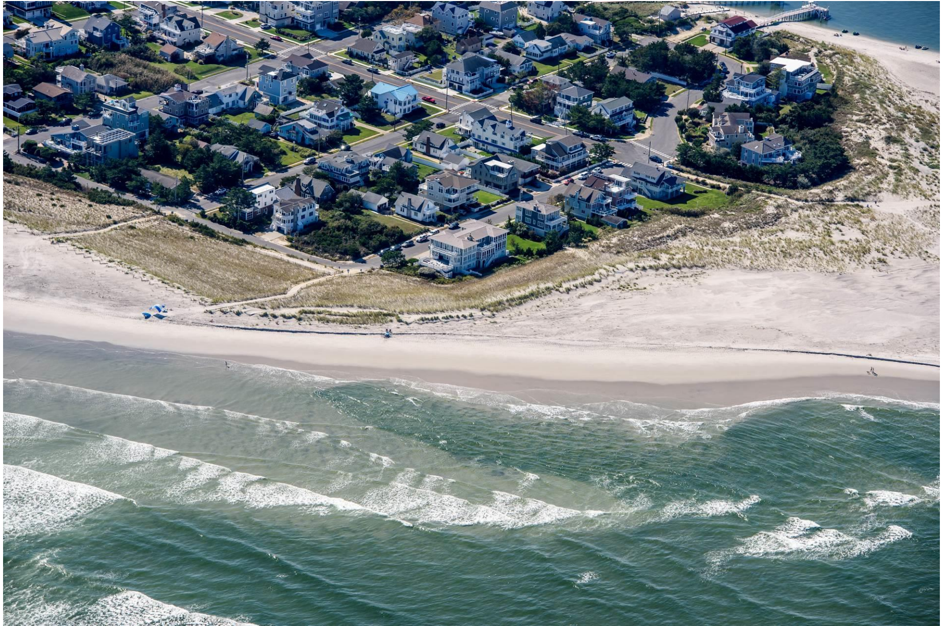
Figure 4. Aerial view of Seaview Avenue profile beach September 25, 2021. While shallow wave-like bars still lie just offshore, the beach berm has been cut into a vertical scarp right at the end of Seaview Avenue and that scarp continues into the NJ State Park land to the northwest. Significant volumes of new sand moving north toward the inlet from the southern bar system is required if the erosion is not to move into the 2019-2020 USACE rebuilt dunes this winter. It is the common combination of the breaking incoming wave angles to the shoreline beach combined with the flood-tidal currents moving into Corson's Inlet that generate rapid sand transfer away from this critical region. The five residential properties north of Seaview Avenue at the park boundary probably represent over $15,000,000 in ratable assets.
