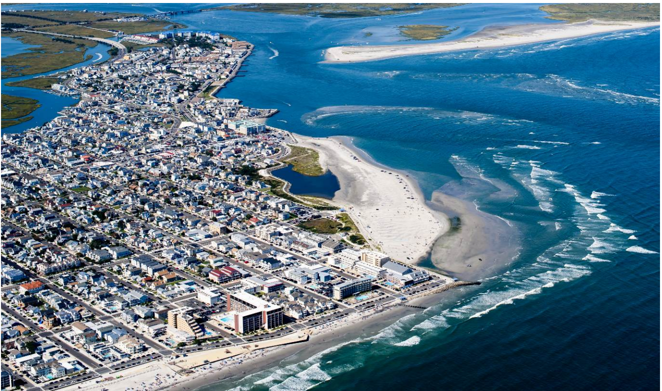
Figure 1. A view along the North Wildwood northern oceanfront and Hereford Inlet shoreline September 25, 2021. The ebb-tidal channel that appeared to be closing at the seaward end as of March 13, 2021 has done so with breaking waves extending northeast from the jetty into the inlet and along the edge of the island shoal's ebb-sand deposit "tail". The inlet cross section starting at the base of the jetty extended almost 2,200 feet into the inlet without the rod holder needing to swim at low tide on October 19, 2021.
