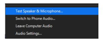
4.) Make sure you can hear the test chime through the classroom speakers and the Zoom speaker is set to the device starting with "DVX." Then, click "Yes."
