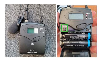
2.) Plug your wired microphone into the "MC/LINE" port and ensure the receiver is not muted.
