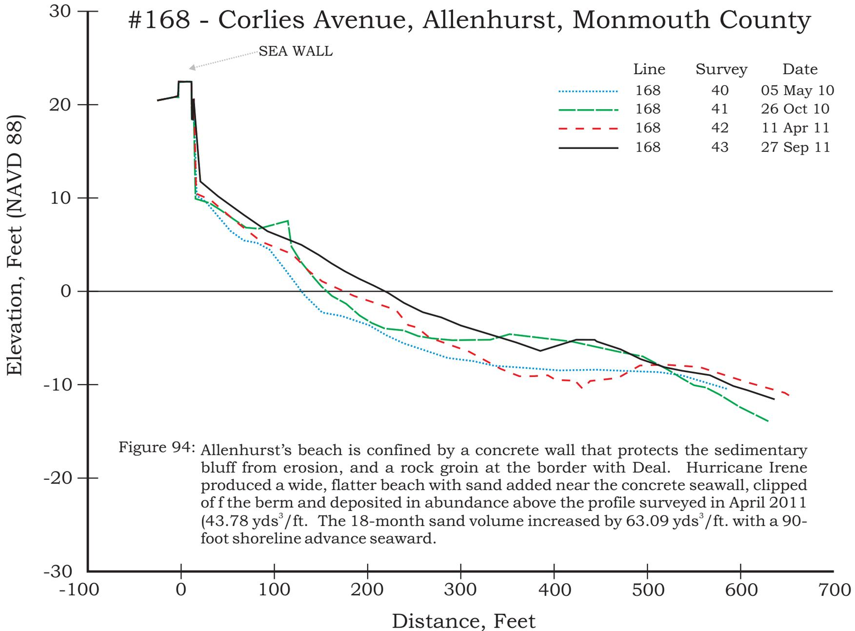
Figure 94: Allenhurst's beach is confined by a concrete wall that protects the sedimentary bluff from erosion, and a rock groin at the border with Deal. Hurricane Irene produced a wide, flatter beach with sand added near the concrete seawall, clipped of f the berm and deposited in abundance above the profile surveyed in April 2011 (43.78 yds<sup>3</sup>/ft. The 18-month sand volume increased by 63.09 yds<sup>3</sup>/ft. with a 90-foot shoreline advance seaward.
