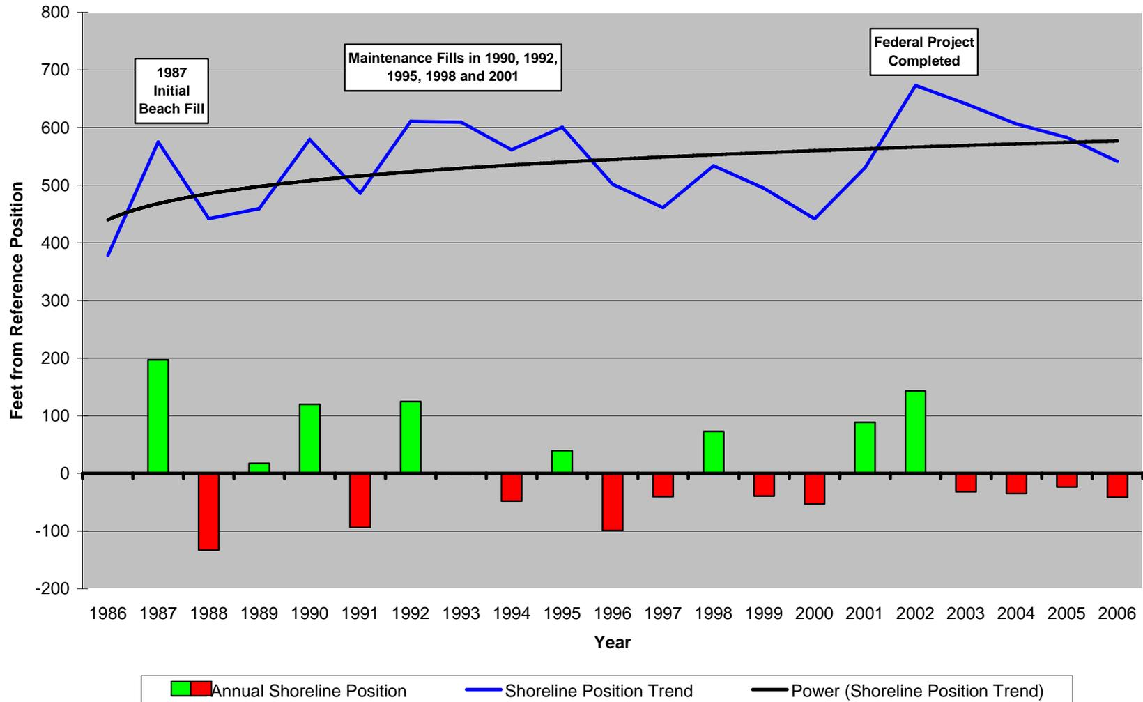
**Figure 170. Site 116.** This site received multiple State and local projects plus a Federal nourishment project between 1987 and 2002. Avalon reacted by pushing forward the NJ State and local sharing work on their northern beaches following serious loss between 1981
