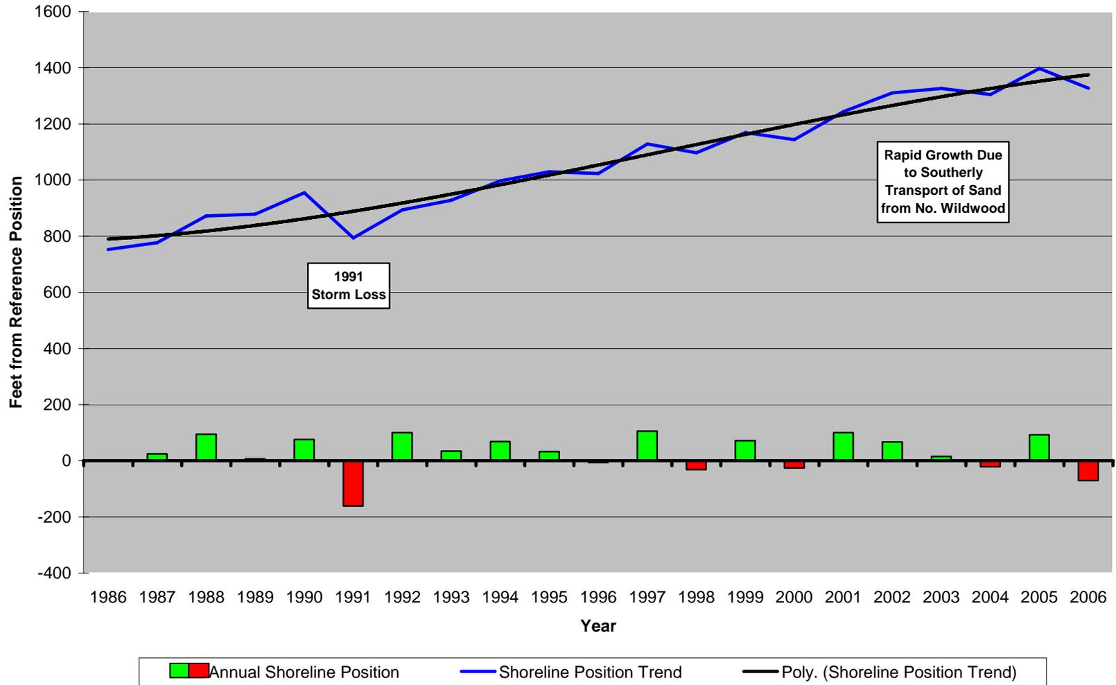
**Figure 182. Site 110.** The trend of retreat dramatically reversed at Cresse Avenue in Wildwood as sand migrated south along the shoreline adding to this beach. The advance amounted to a move from 752 to 1,327 feet seaward of the reference (575 feet). This amounts to about half the sand volume loss at 15<sup>th</sup> Street in N. Wildwood.
