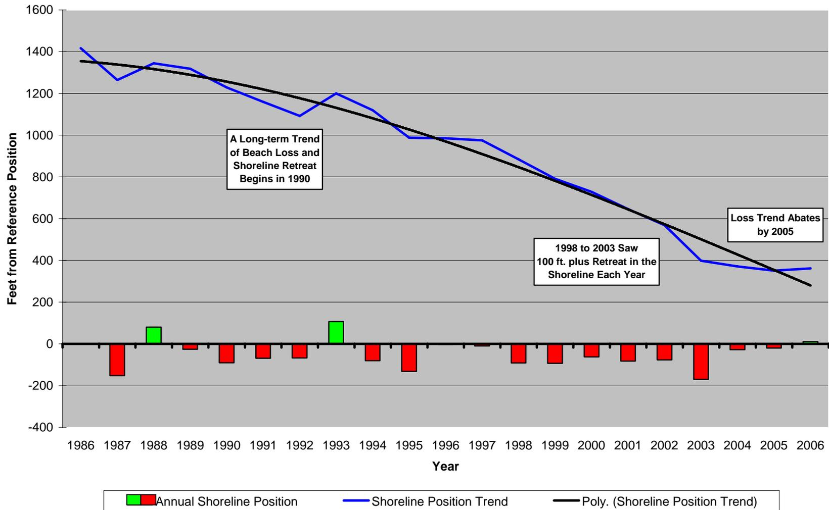
**Figure 180. Site 111.** North Wildwood takes the prize as the most erosional location in New Jersey, the opposite of site 245 in Barnegat Light Borough where the Barnegat Inlet jetty causes the greatest shoreline advance. The initial shoreline position was
