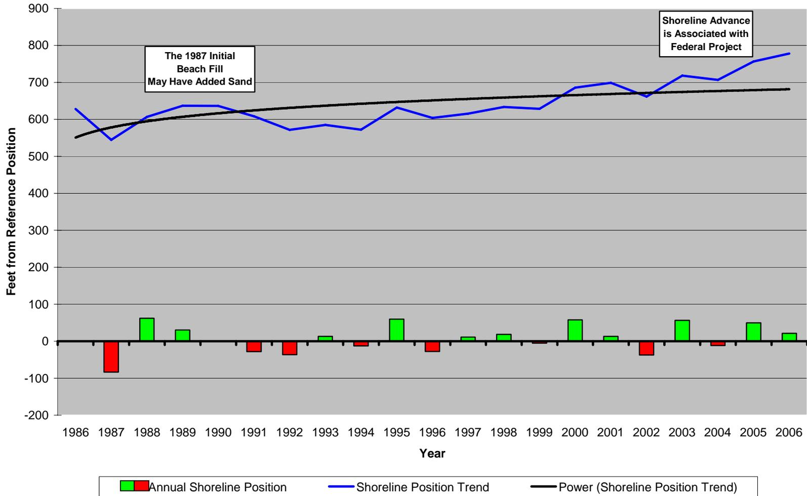
**Figure 174. Site 114.** The trend of shoreline advance continued south from 35<sup>th</sup> Street to include the beach at 70<sup>th</sup> Street in Avalon. No direct placement of sand occurred anywhere between 35<sup>th</sup> and 70<sup>th</sup> Streets, yet the shoreline continued to advance and sand accumulated.
