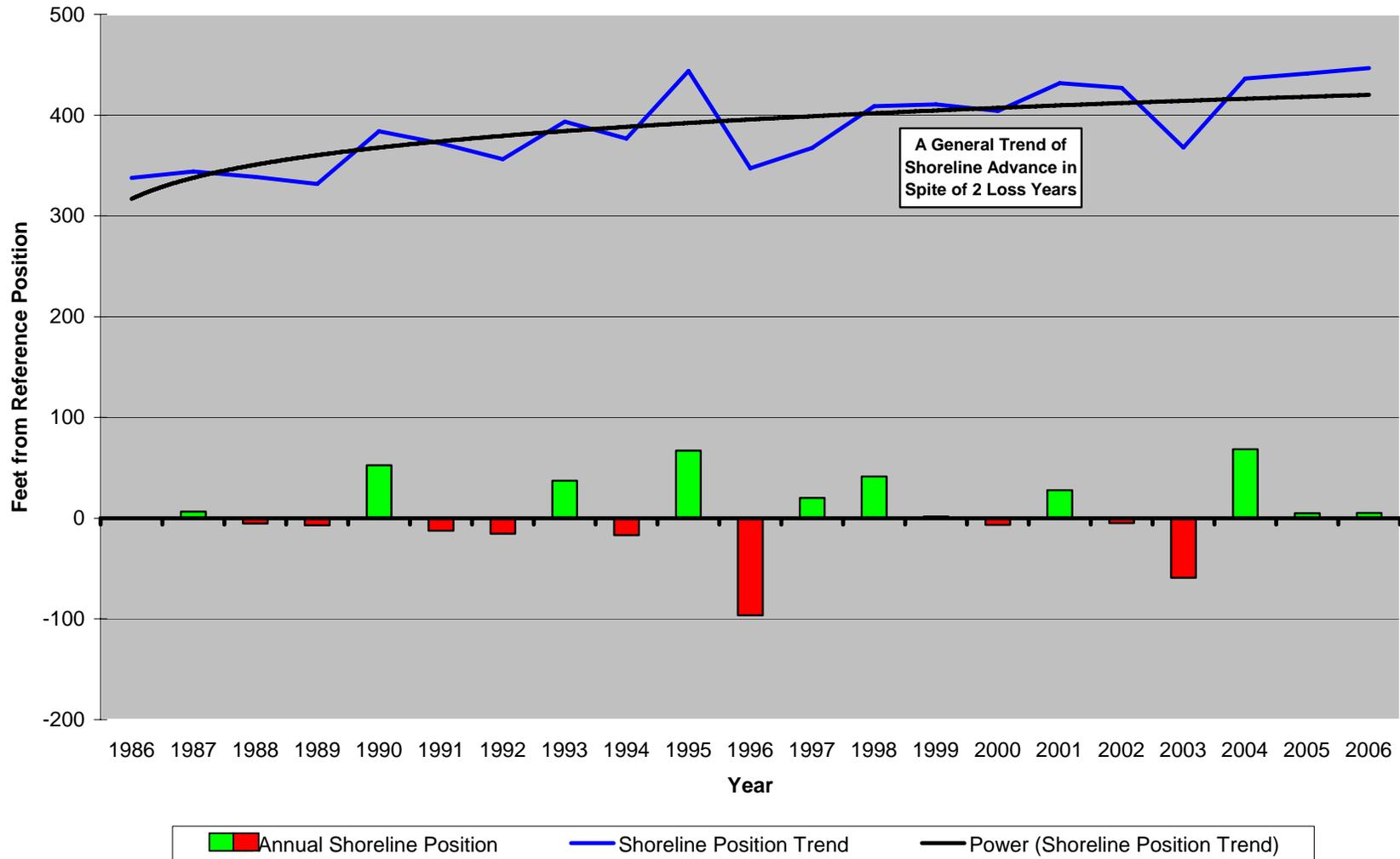
**Figure 162. Site 119.** Toward the middle of Ludlam Island a gradual trend of shoreline advance has occurred in spite of two years of considerable retreat. The shoreline position has moved seaward by 100 feet in 20 years.
