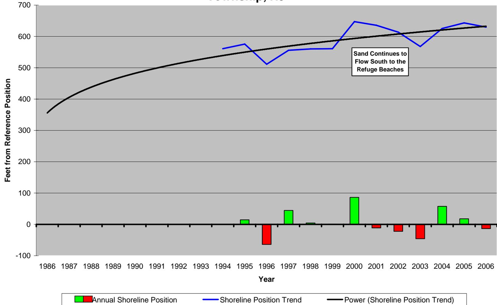
**Figure 186. Site 208.** Established within the natural area of the Cape May National Wildlife Refuge in 1994, this site shows the impact of the 1911-vintage Cold Springs Inlet jetties in trapping sand. The area has been constructional for decades.
