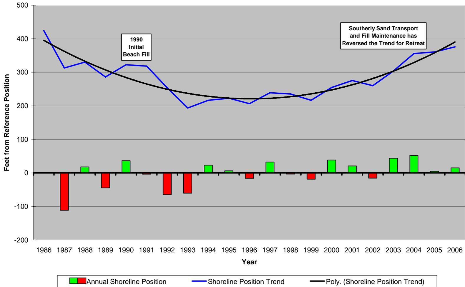
**Figure 192. Site 206.** Broadway Avenue lies just a short distance from the Cape May City boundary with an undeveloped segment of the shoreline known as Cape May Meadows. A rock groin was put in place to retain sand on the municipal beach years prior to
