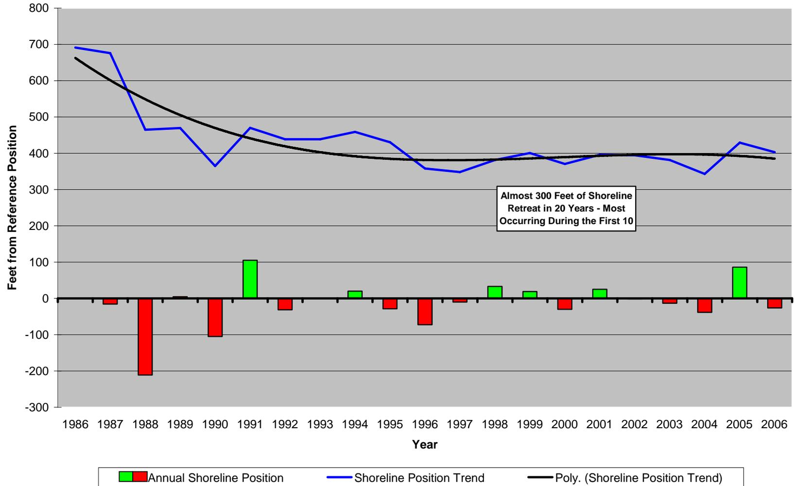
**Figure 202. Site 101.** Large shoreline changes occurred prior to 1996 with only one year with an advance (1991). The post 1996 performance was nearly level with little change noted. The net change was nearly 300 feet over 20 years.
