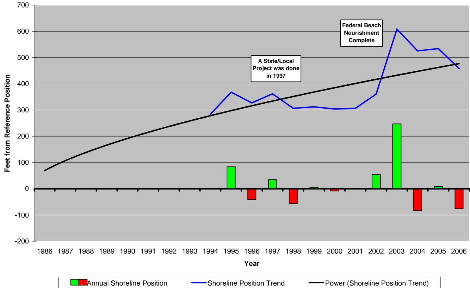
**Figure 178. Site 212.** Inserted into the rotation of survey sites in 1994 to get data close to Hereford Inlet, this site also shows the impact of the Federal project completed in 2003. Similar losses at this location have cut back the total volume as the shoreline
