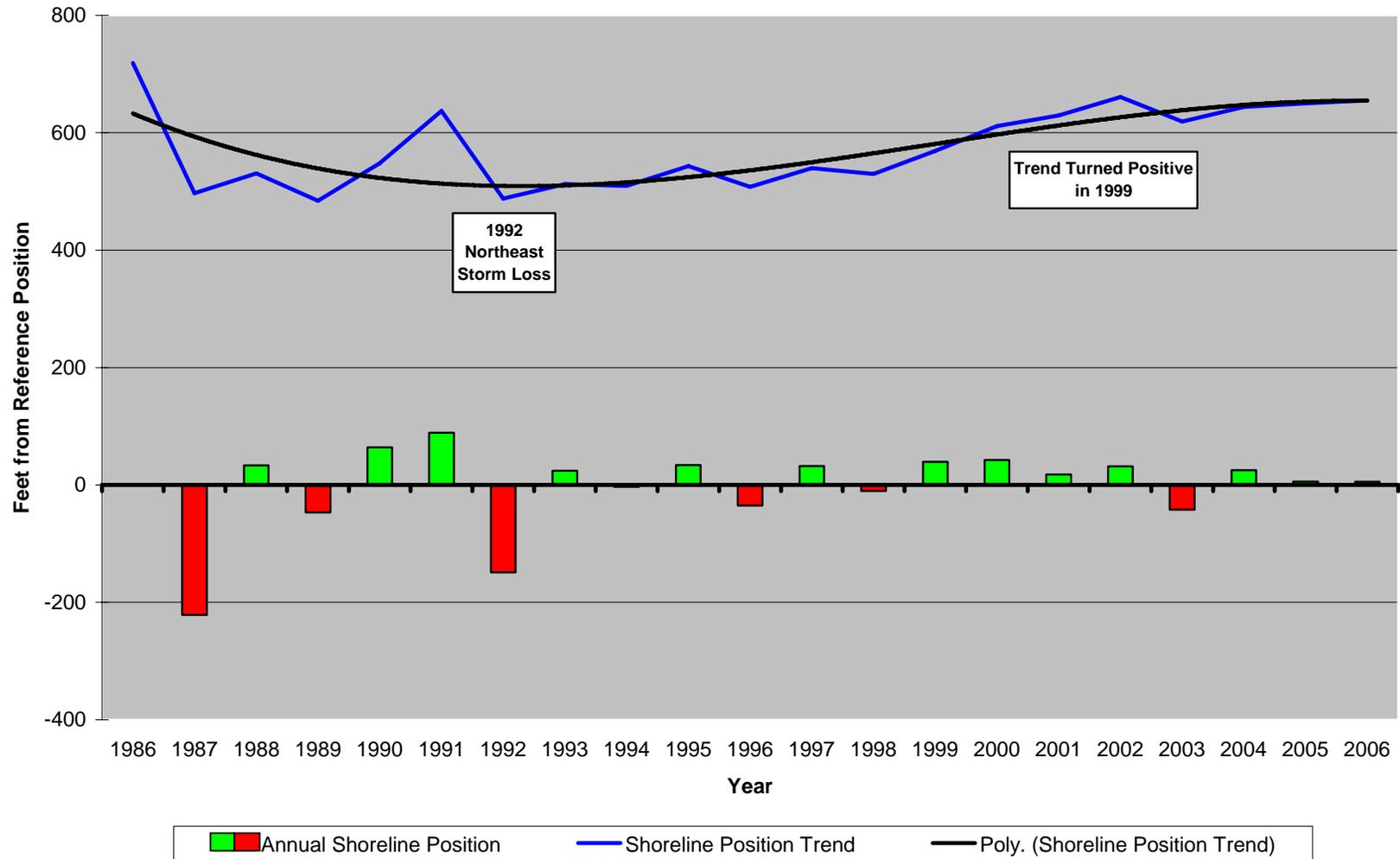
**Figure 184. Site 109.** A trend of storm-related loss pushed the shoreline about 200 feet landward by 1992. This was followed by a trend of advance that continued from 1993 to 2006. No beach material was pumped onto any of this shoreline.
