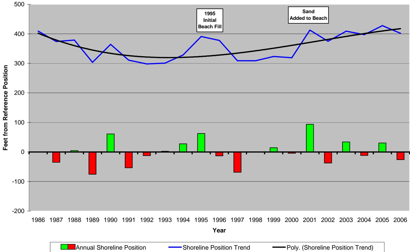
**Figure 156. Site 122.** At the south end of Pecks Beach the State of NJ assumed the role of cooperative partner in beach restoration. The fill first arrived in 1995 adding substantially to the width of the beach. Since then there has been slow accretion combined with shoreline advance to 2005. The trend line shows the turn-around in shoreline position.
