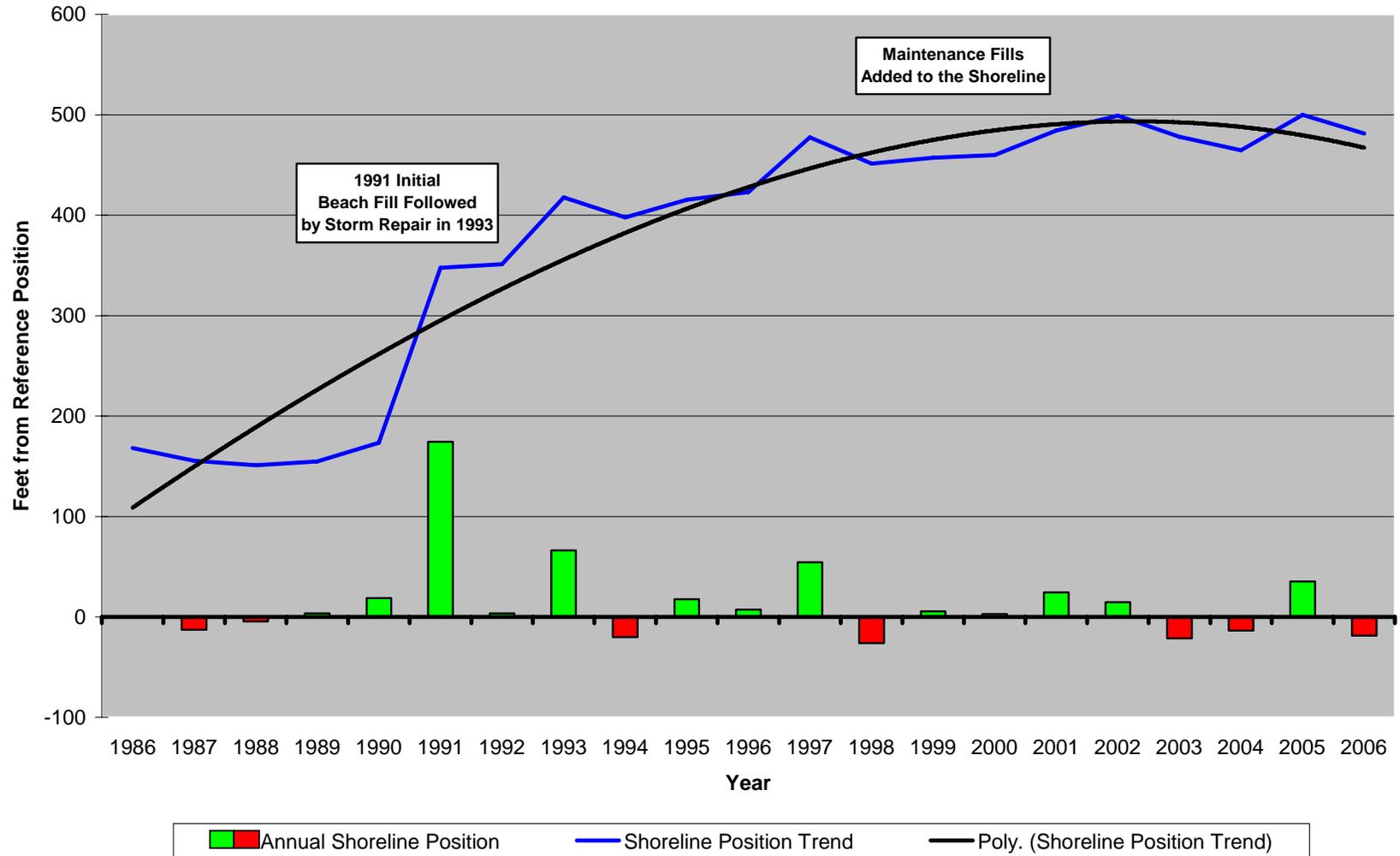
**Figure 190. Site 107.** Baltimore Avenue beach was wet sand at the base of the rock revetment along Beach Drive in 1986 to 1990 prior to the Federal project’s commencement. Sand was added multiple times starting in 1993 principally as a result of damage done
