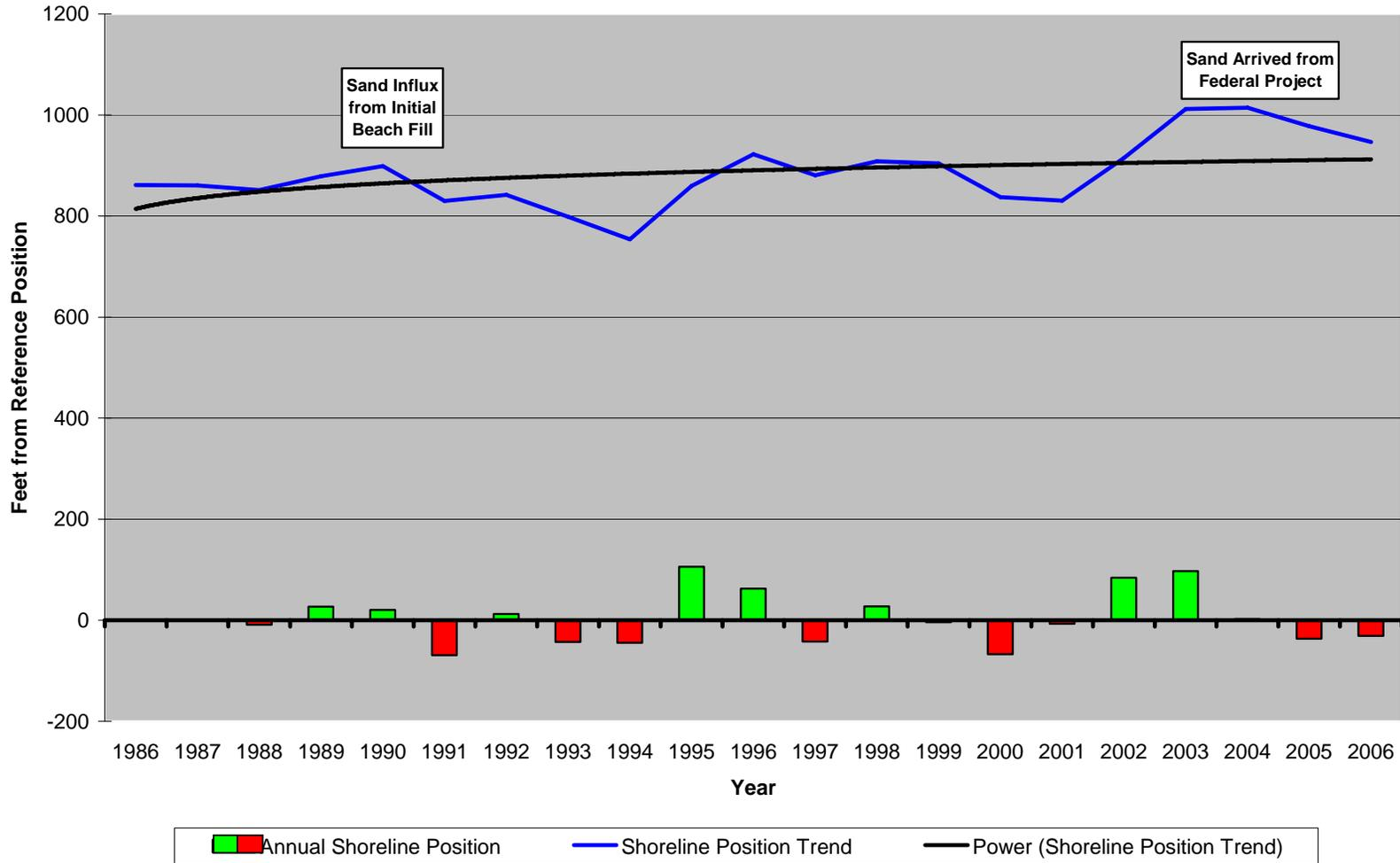
**Figure 172. Site 115.** Beginning at 35<sup>th</sup> Street, the Avalon shoreline has been steadily accumulating sand producing a steady advance in the shoreline position. There have been no direct placements of sand along this beach, but littoral transport has moved material into position here over the past two decades.
