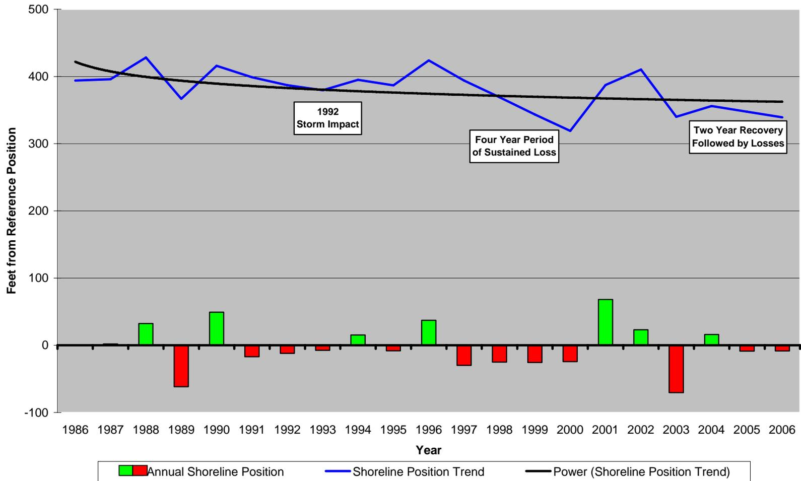
**Figure 160. Site 120.** No sand has been added to this shoreline reach except for dune reconstruction following several northeasters. After these storm episodes, quarry sand was used to cover the core of the dune. The beach is low and narrow making it subject to frequent storm overwash episodes. The trend is one of retreat over the past 20 years.
