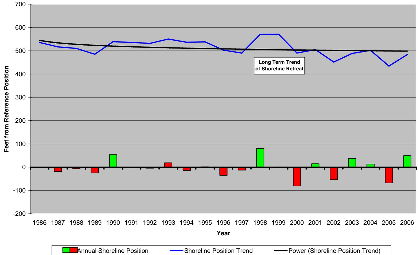
**Figure 164. Site 118.** The shoreline position trend saw a minor retreat at 57<sup>th</sup> Street in Sea Isle City. The beach has not had nourishment sand applied since 1978, which was prior to NJ Beach Profile surveying.
