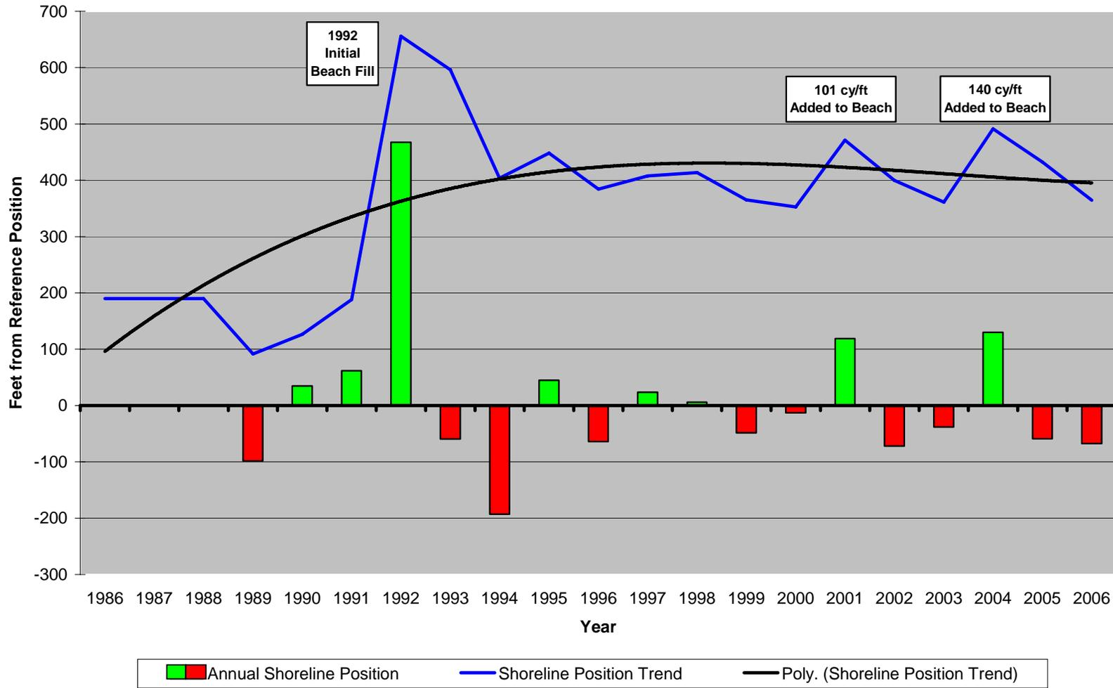
**Figure 150. Site 125.** This site in Ocean City has suffered from chronic losses since beach nourishment under either State or Federal projects commenced in 1983. Ocean City’s beach restoration using sand from the bays goes back to 1952 when the ACOE undertook
