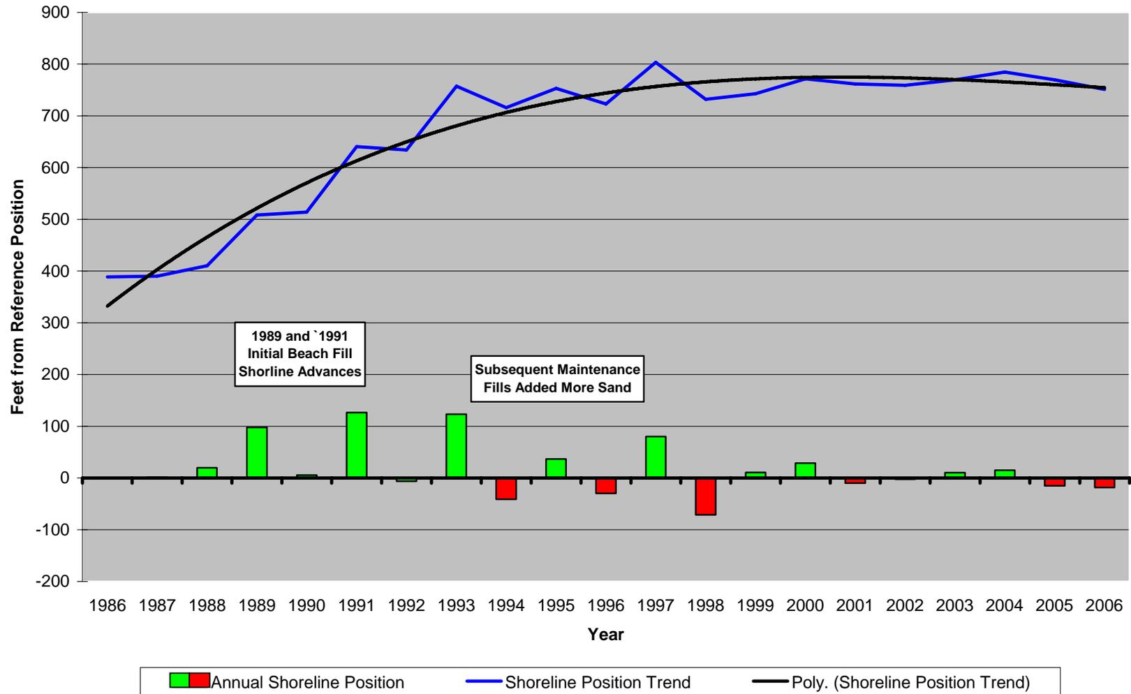
**Figure 188. Site 108.** The City of Cape May enjoyed the benefits of the initial Federal project constructed by the Philadelphia District on the NJ coastline. The trend line represents the addition of sand in 1989 through 1997 with direct placement at this site.
