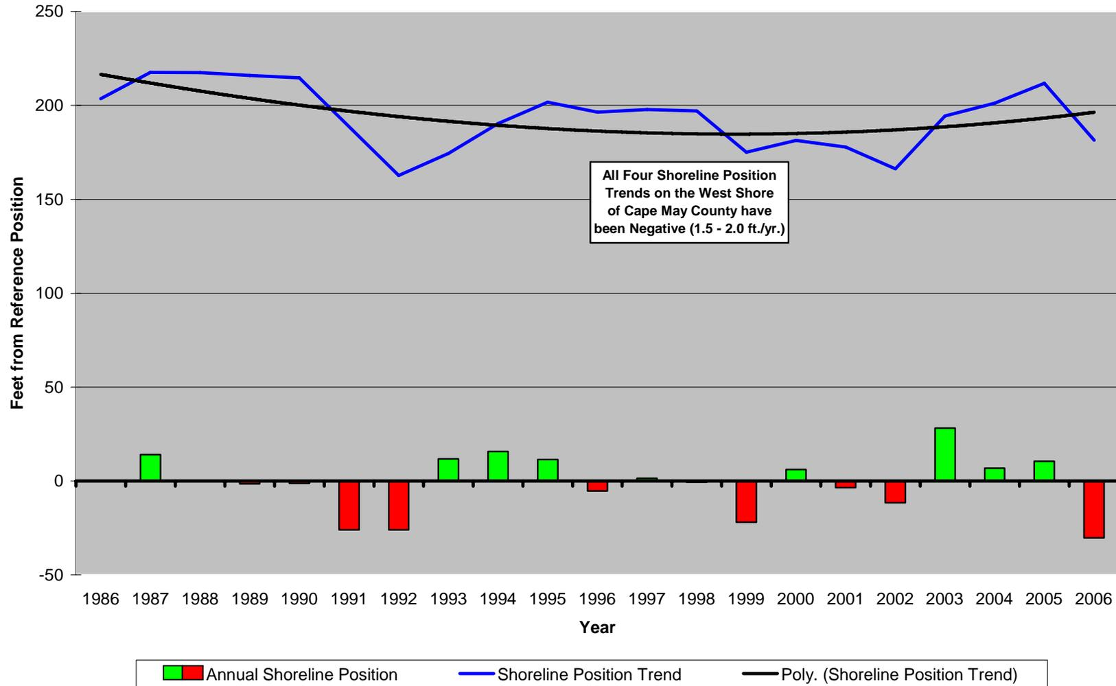
**Figure 200. Site 102.** The negative shoreline trend was less at Whittier Avenue in North Cape May, but still in the range of 1.5 to 2.0 feet per year. This corresponds to rates determined earlier when the NJDEP historical shoreline mapping program was completed
