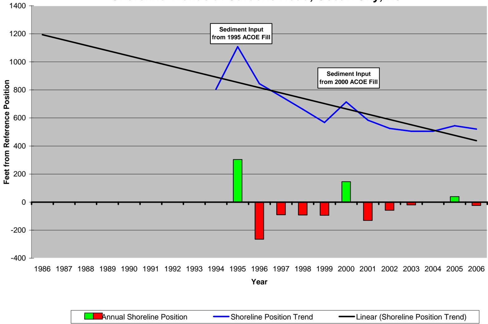
**Figure 148 – Site 225.** This site was established in 1994 to provide information near Great Egg Inlet. This profile line is strongly influenced by sand placement events on the oceanfront beach. During the years following the sand placement, the beach expanded as
