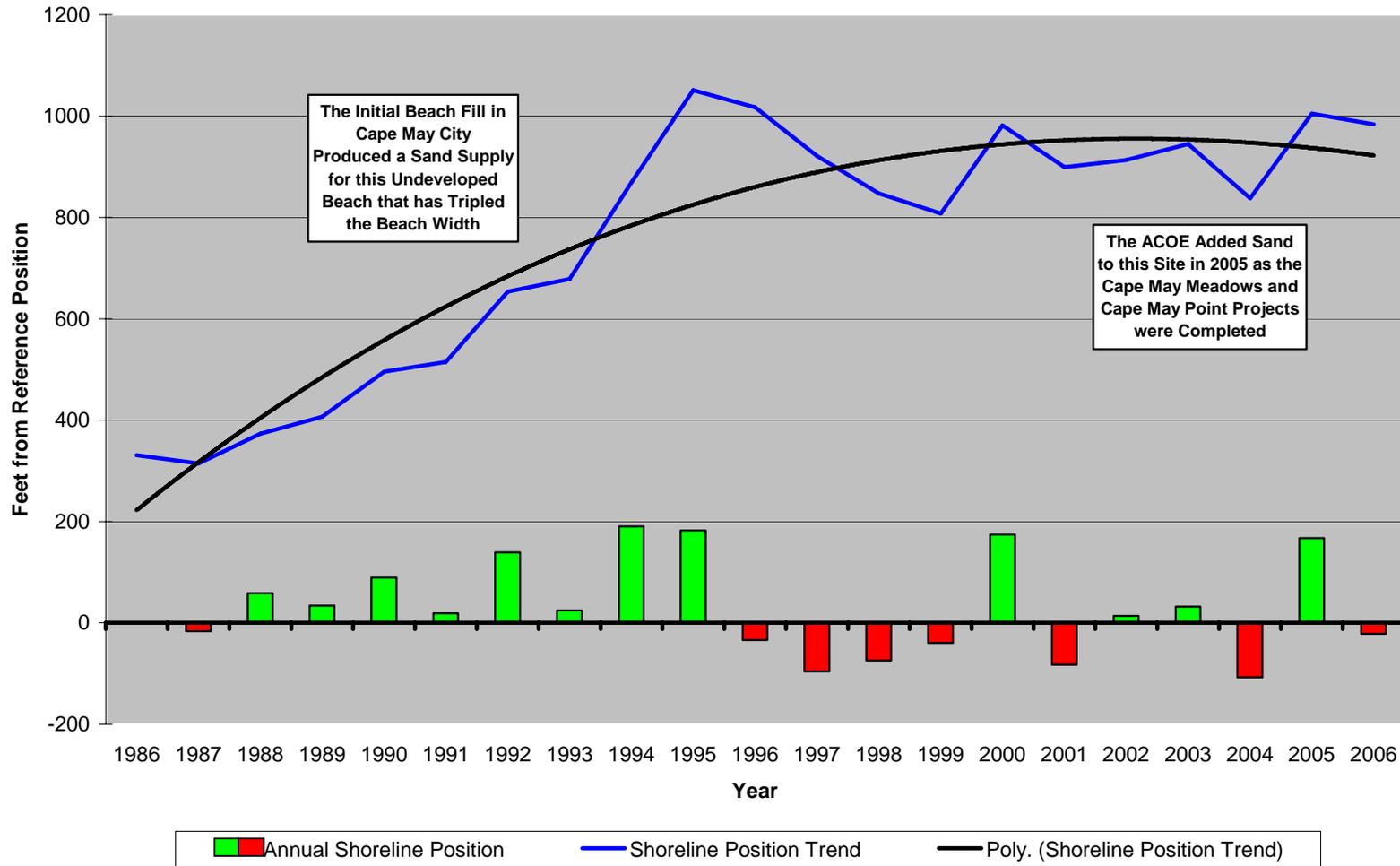
**Figure 194. Site 105.** Located on the opposite side of the Cape May City groin from the Broadway Avenue site, this location documents the large-scale sediment transport around this groin onto the undeveloped beaches of the Cape May Meadows. The State
