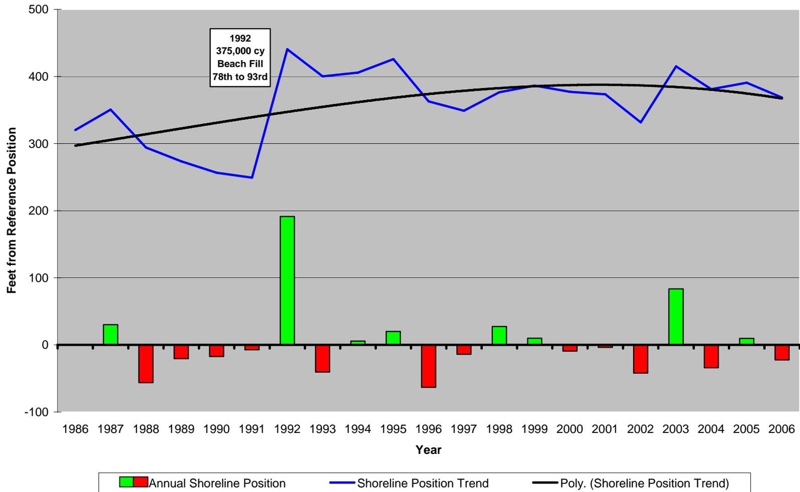
**Figure 166. Site 117.** In 1992 Sea Isle City conducted a beach nourishment project between 78<sup>th</sup> Street and Townsends Inlet. The impact on the shoreline position is clear as the shoreline position moved 211 feet seaward. Modest retreat followed in a non-linear fashion over the next 14 years.
