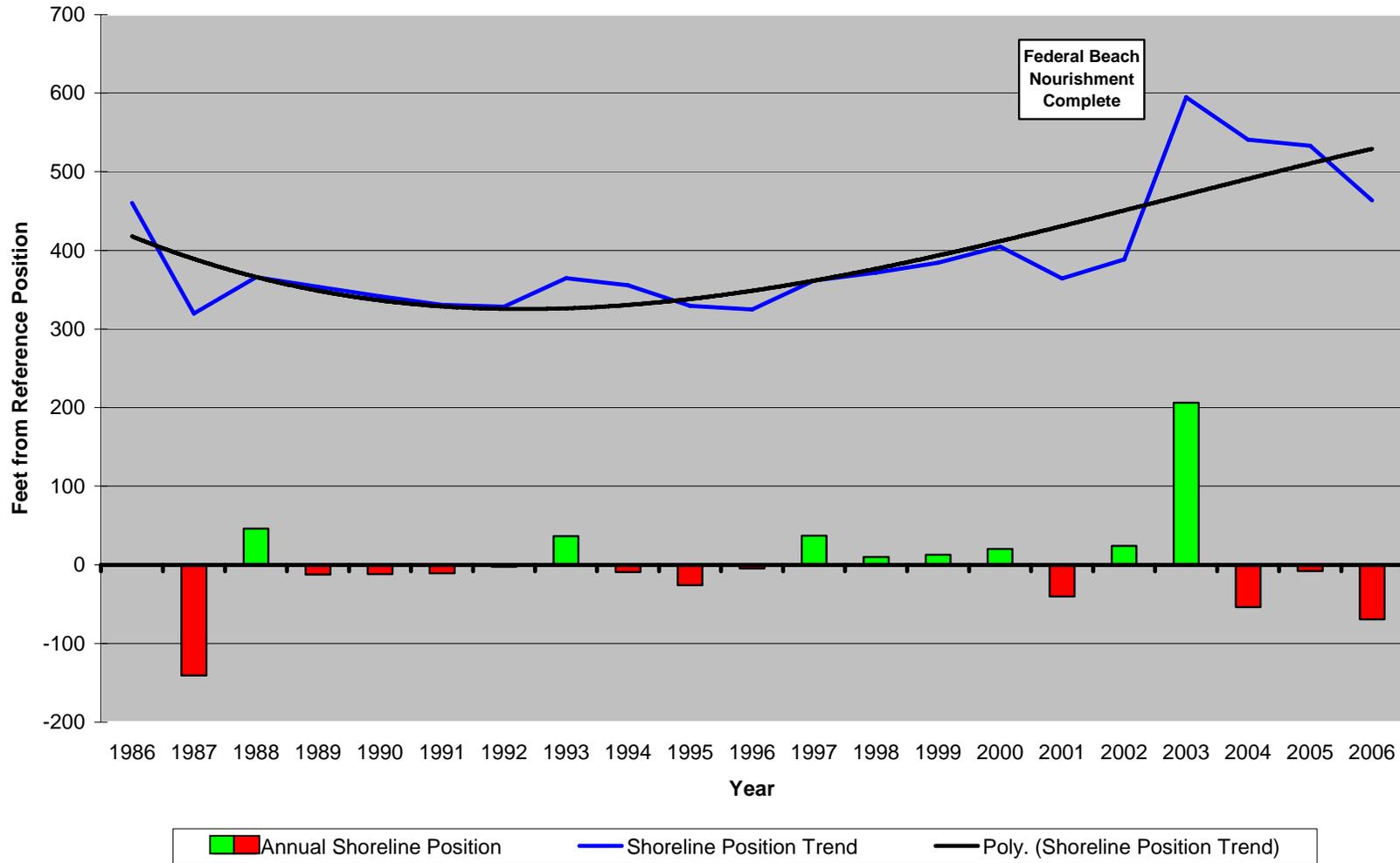
**Figure 176. Site 113.** The Borough of Stone Harbor conducted its own beach nourishment project in 1997 to counter a long trend of erosion that had pushed the dune back landward of the bulkhead along the central segment of the municipal beach. In 2003, the
