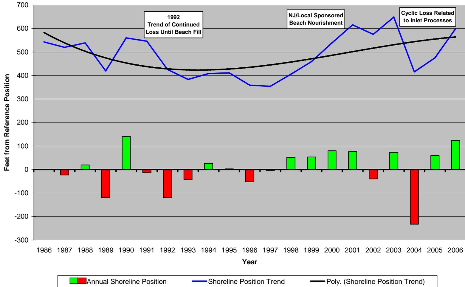
**Figure 158. Site 121.** Positioned near Corson’s Inlet, this site shows the influence that both beach nourishment and inlet dynamics can have on an area. Sand naturally cycles between the inlet channel, the ebb-tidal shoals and the beach creating episodes of extensive
