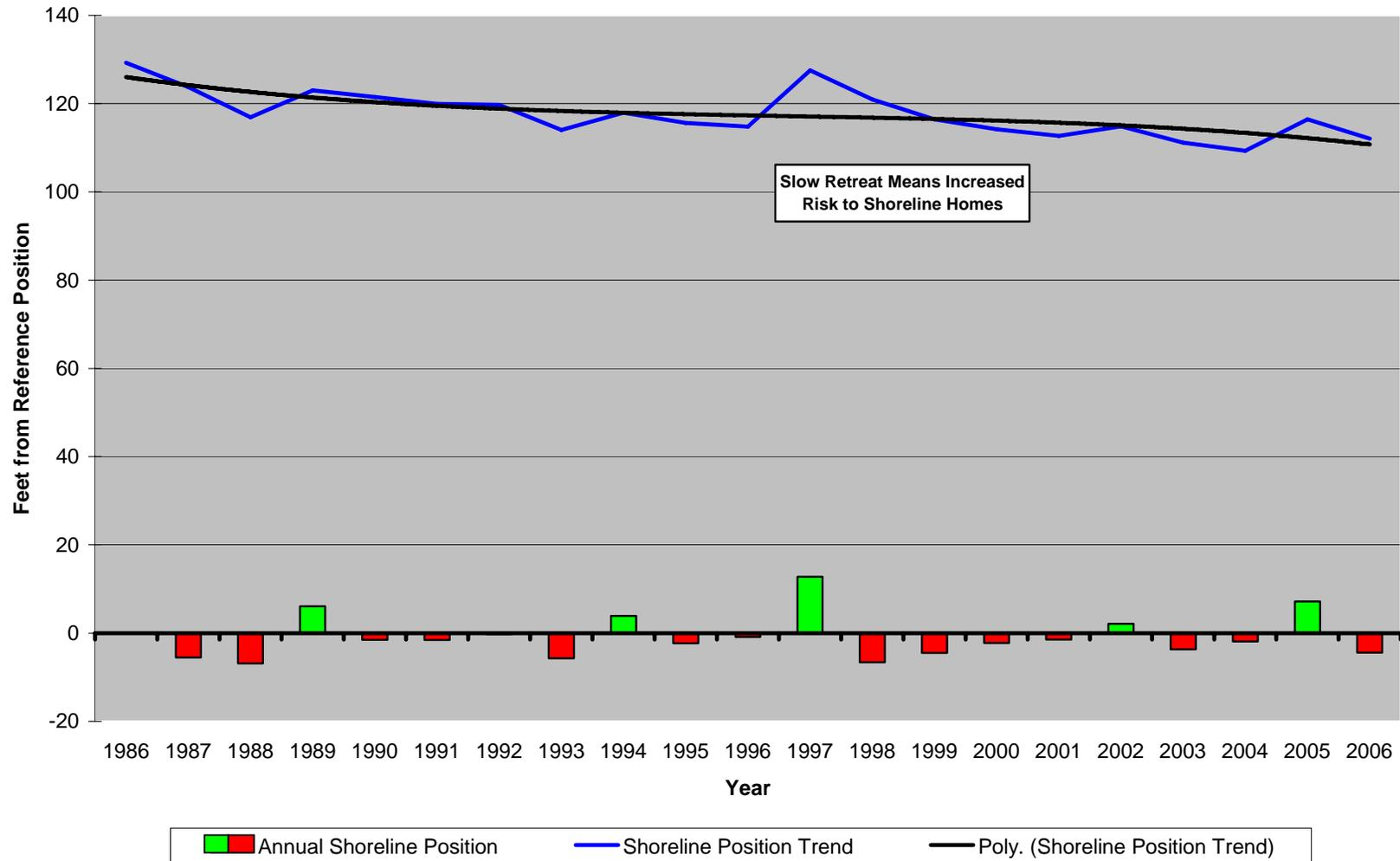
**Figure 204. Site 100.** The northern most NJBPN site in Delaware Bay lies just south of Bidwell Creek at the terminus of continuous sandy beach shorelines in the Bay. Slow, steady shoreline retreat has produced enough retreat to endanger homes built on the
