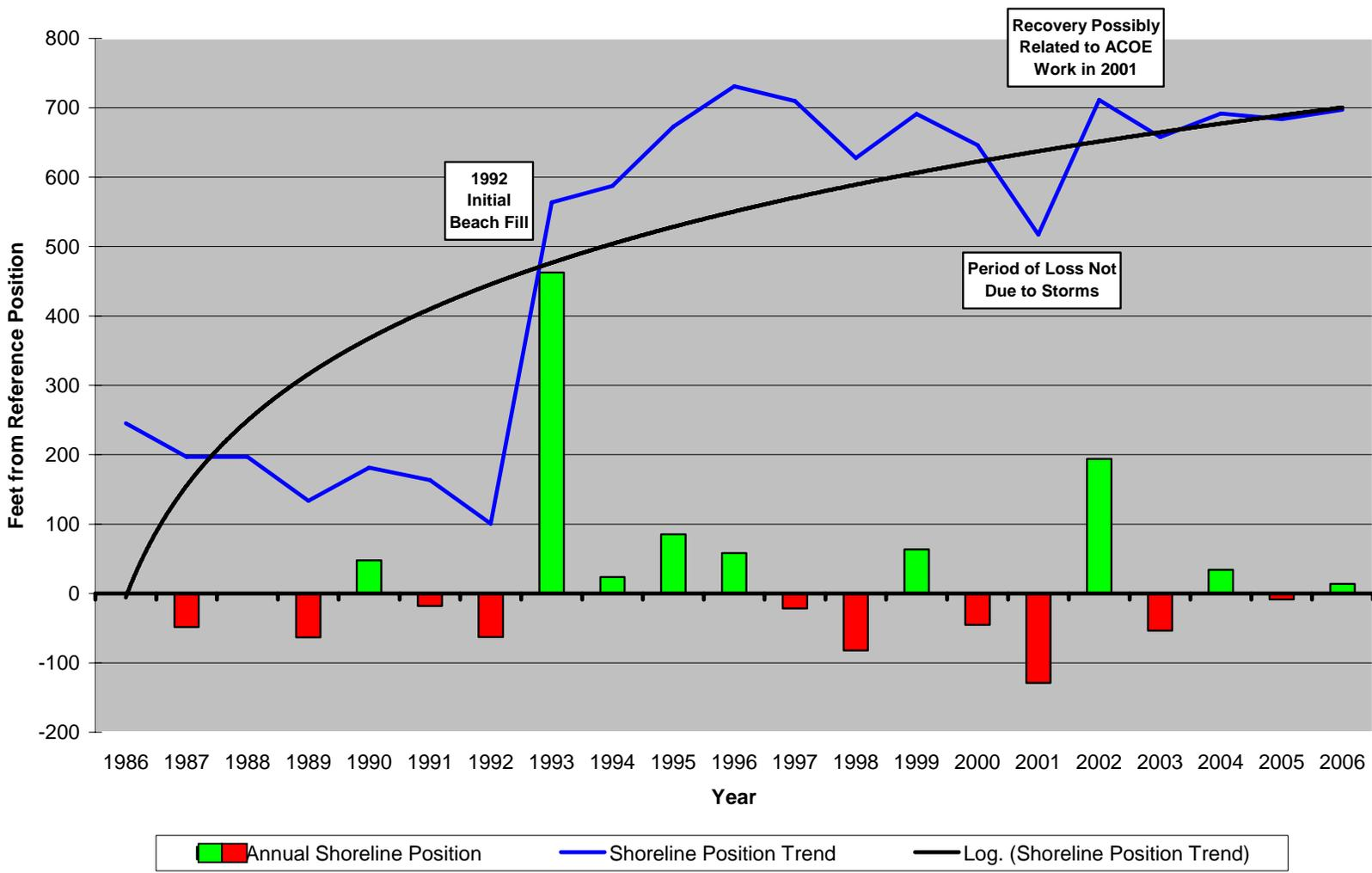
**Figure 152. Site 124.** Further south along the Ocean City shoreline, the beach has responded dramatically different from that seen at 6<sup>th</sup> Street in Ocean City. The decline in beach width was evident between 1986 and 1992 when the initial fill commenced at this site.
