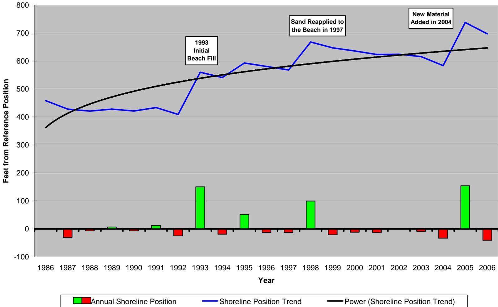
**Figure 154. Site 223.** Prior to the commencement of beach nourishment, 34<sup>th</sup> Street showed minor declines in shoreline position. Response to each beachfill activity produced a step seaward in the position of the shoreline moving the zero elevation location 300
