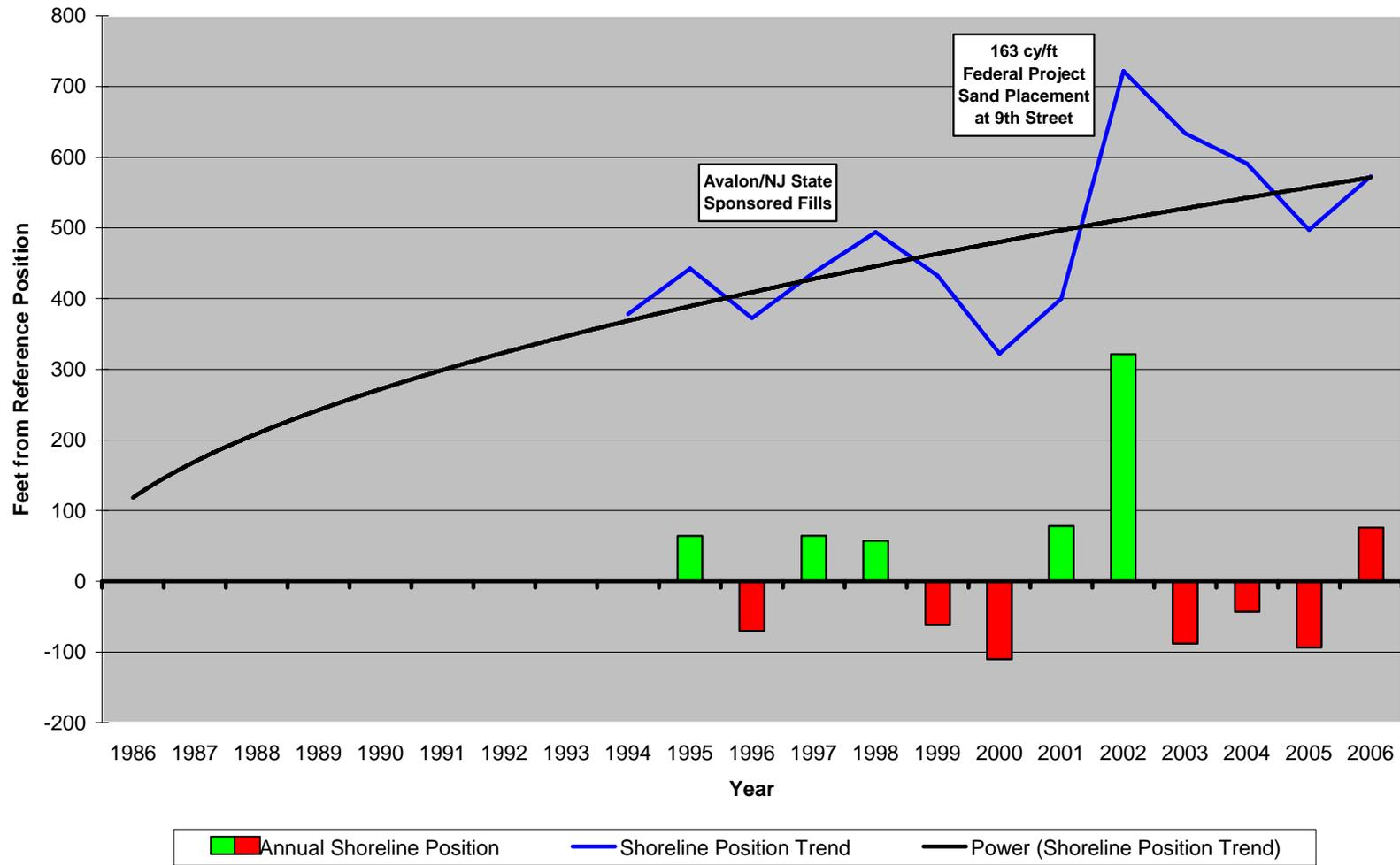
**Figure 168. Site 216.** Established in 1994 to study the inlet-associated shoreline south of Townsends Inlet, 9<sup>th</sup> Street has responded to beach nourishment multiple times. The largest spike in shoreline advance seaward came in 2002 when the Federal project was complete.
