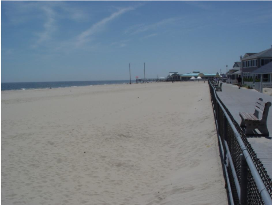
Figure 108. The beach along much of Point Pleasant Beach has no dune because the community leaders desire a unobstructed view of the ocean beach from the boardwalk and the large number of summer beach visitors. This series of profiles has resulted in expanded berm growth between each pair of surveys. The distance from the boardwalk to the berm crest increased by 100 feet during the 18-month study period, the majority occurring between March and October 2007.
