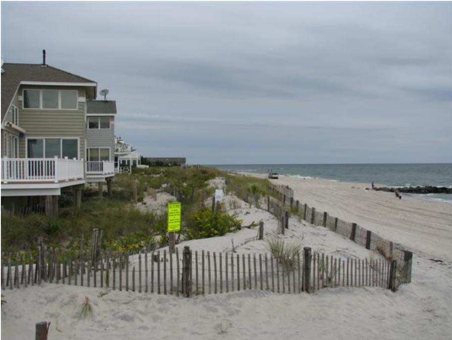
By October 6th 2008 some vegetation has invaded the new sand deposited among the three fences, but no sizable growth is evident. The net change was a gain of 7.18 yds<sup>3</sup>/ft., but with a 4-foot shoreline retreat. This reflects stability at this site.
