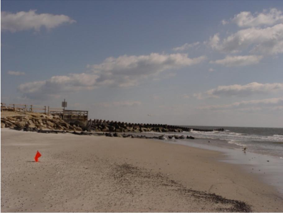
On March 5th 2007 this view toward the terminal groin shows a narrow beach with considerable exposure of the rocks. Northeast storms act to move sand around this groin where post-storm waves move it onto the beach after the storm. In the absence of northeasters sand will move up the beach from the south if southeast wave conditions prevail for extended periods of time.
