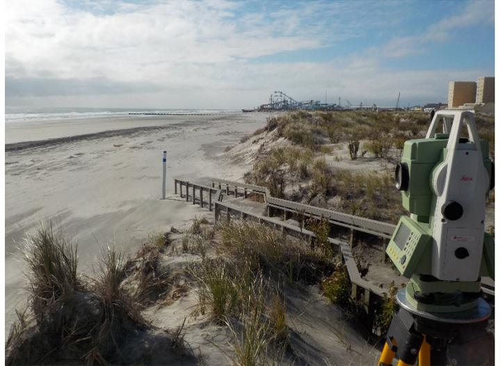
The 15<sup>th</sup> Avenue site is just south of the locus of major erosion problems in North Wildwood. The March 18, 2016 view to the left shows storm debris deposited at the toe of the dune with a dry beach pocket remaining near 20<sup>th</sup> Avenue to the south. By November 15, 2017 the situation had improved a bit with a wider beach, but note that some dune retreat had occurred (distance from the white pole to the dune slope).
