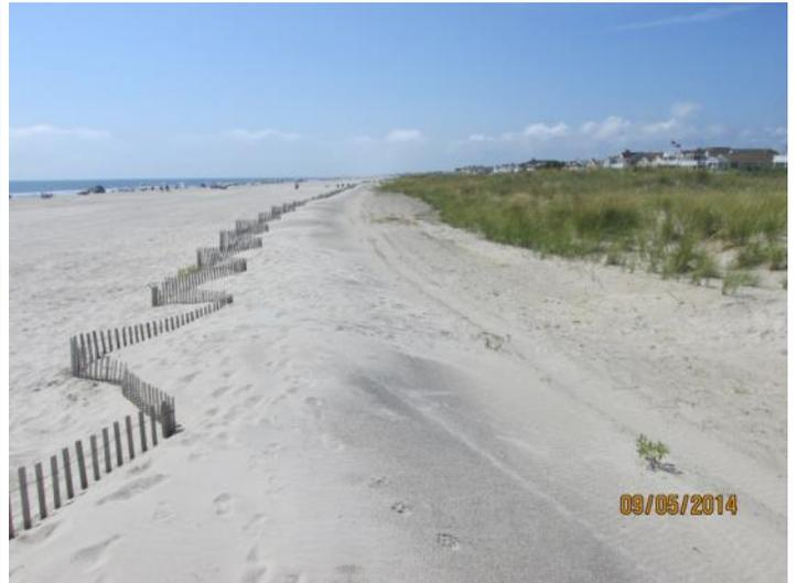
In the October 18, 2013 photo (left), sand piles returned to the beach from inland following Sandy were spread to support incipient dune growth. The right hand view on September 5, 2014 shows significant wind accumulation landward of the sand fencing and a beach with a moderate addition of sand at the berm.
