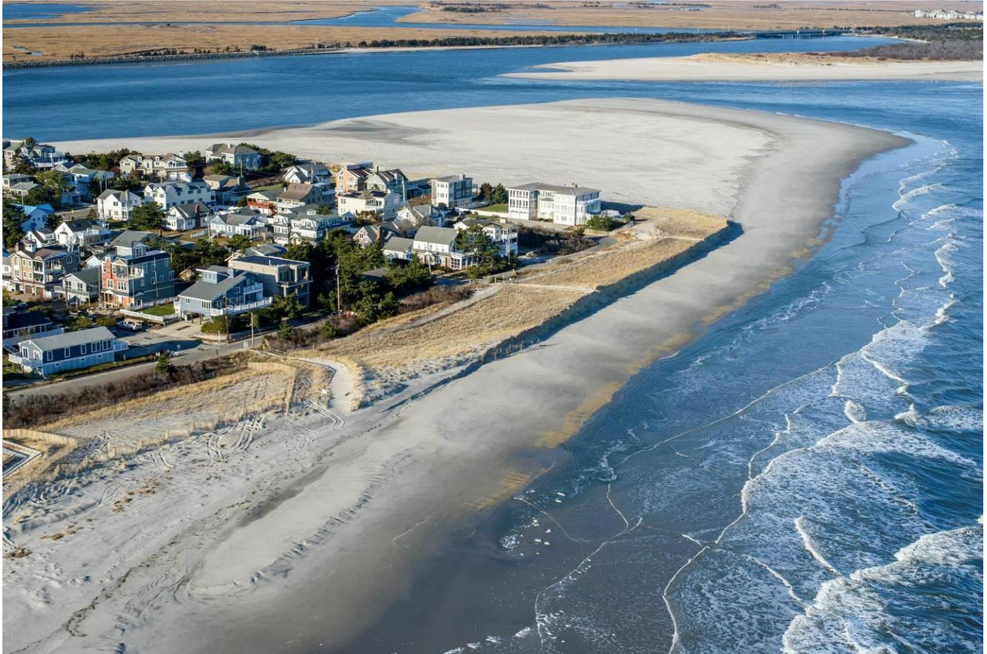
*Above is an aerial view of Strathmere, taken December 11, 2018, showing the relationship between the shoreline orientation between Williams Avenue and the tip of the sand spit in the inlet. This alignment is currently truncating the dune between its northern end and Seacliff Avenue. This time, there does not appear to be a subsidiary ebb-tidal channel causing this erosion. (Photo by Ted Kingston).*
