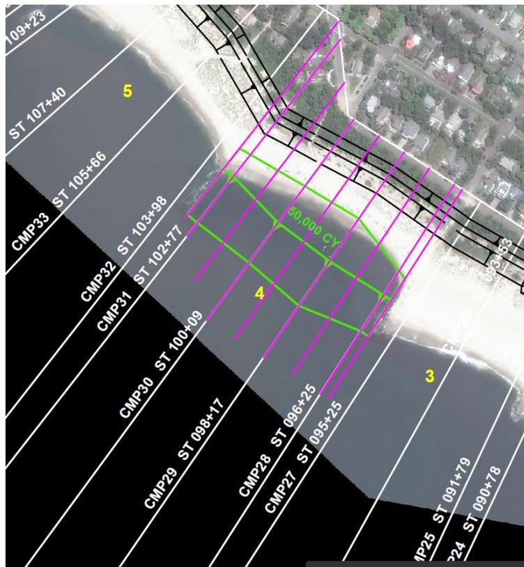
**Figure 1. Site plan for the USACE beach maintenance completed at Lake Drive, Cape May Point as of February 2021 adding 50,000 cubic yards of sand derived from the NJ State Park beach and truck hauled to Lake Drive.**
