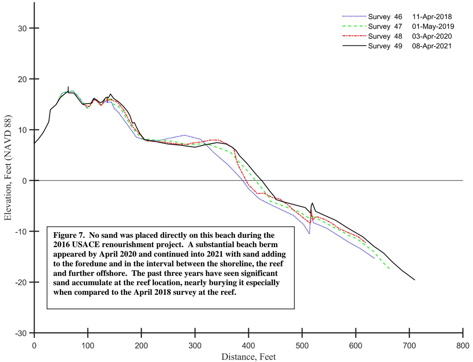
**Figure 7. No sand was placed directly on this beach during the 2016 USACE renourishment project. A substantial beach berm appeared by April 2020 and continued into 2021 with sand adding to the foredune and in the interval between the shoreline, the reef and further offshore. The past three years have seen significant sand accumulate at the reef location, nearly burying it especially when compared to the April 2018 survey at the reef.**
