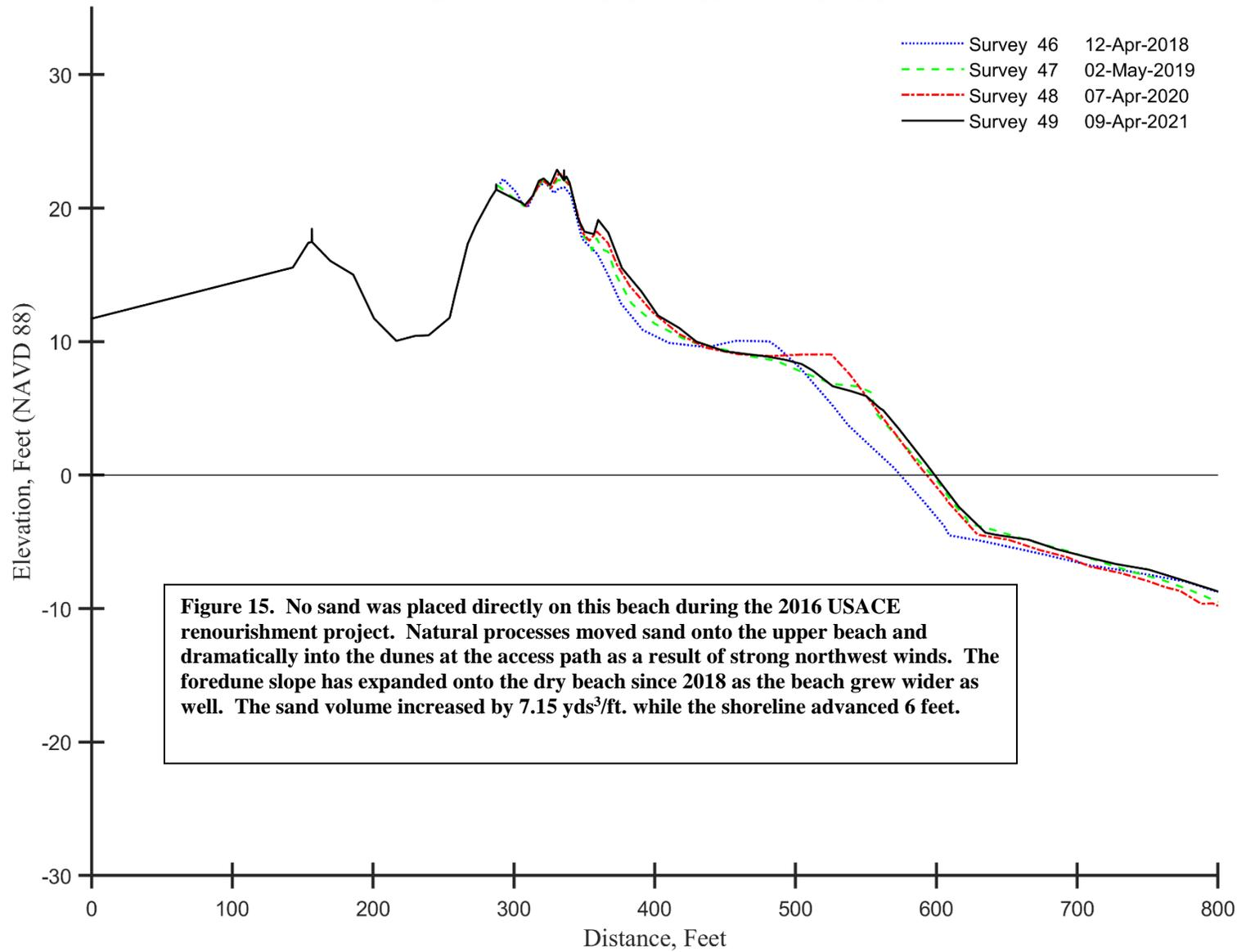
**Figure 15. No sand was placed directly on this beach during the 2016 USACE renourishment project. Natural processes moved sand onto the upper beach and dramatically into the dunes at the access path as a result of strong northwest winds. The foredune slope has expanded onto the dry beach since 2018 as the beach grew wider as well. The sand volume increased by 7.15 yds<sup>3</sup>/ft. while the shoreline advanced 6 feet.**
