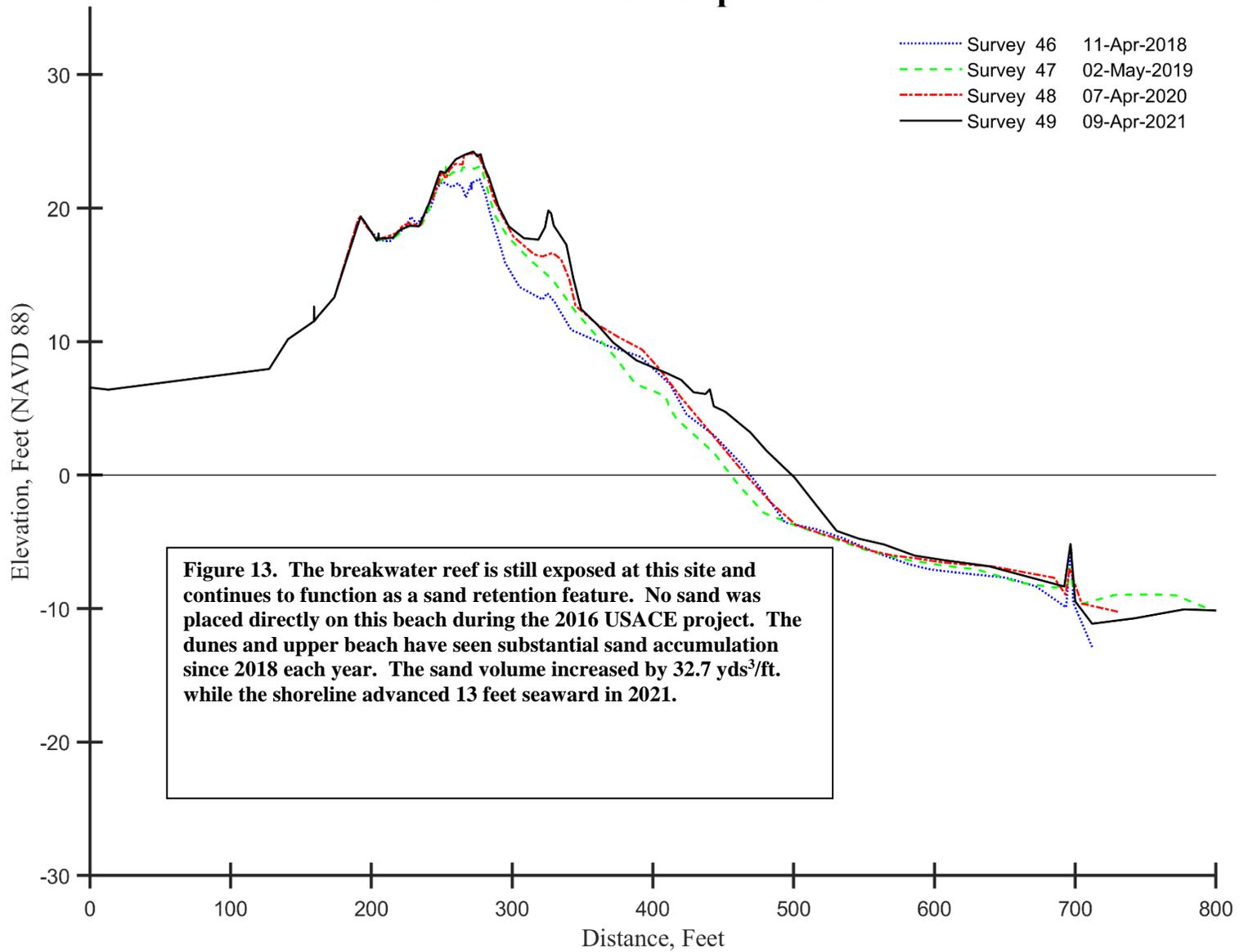
**Figure 13. The breakwater reef is still exposed at this site and continues to function as a sand retention feature. No sand was placed directly on this beach during the 2016 USACE project. The dunes and upper beach have seen substantial sand accumulation since 2018 each year. The sand volume increased by 32.7 yds<sup>3</sup>/ft. while the shoreline advanced 13 feet seaward in 2021.**
