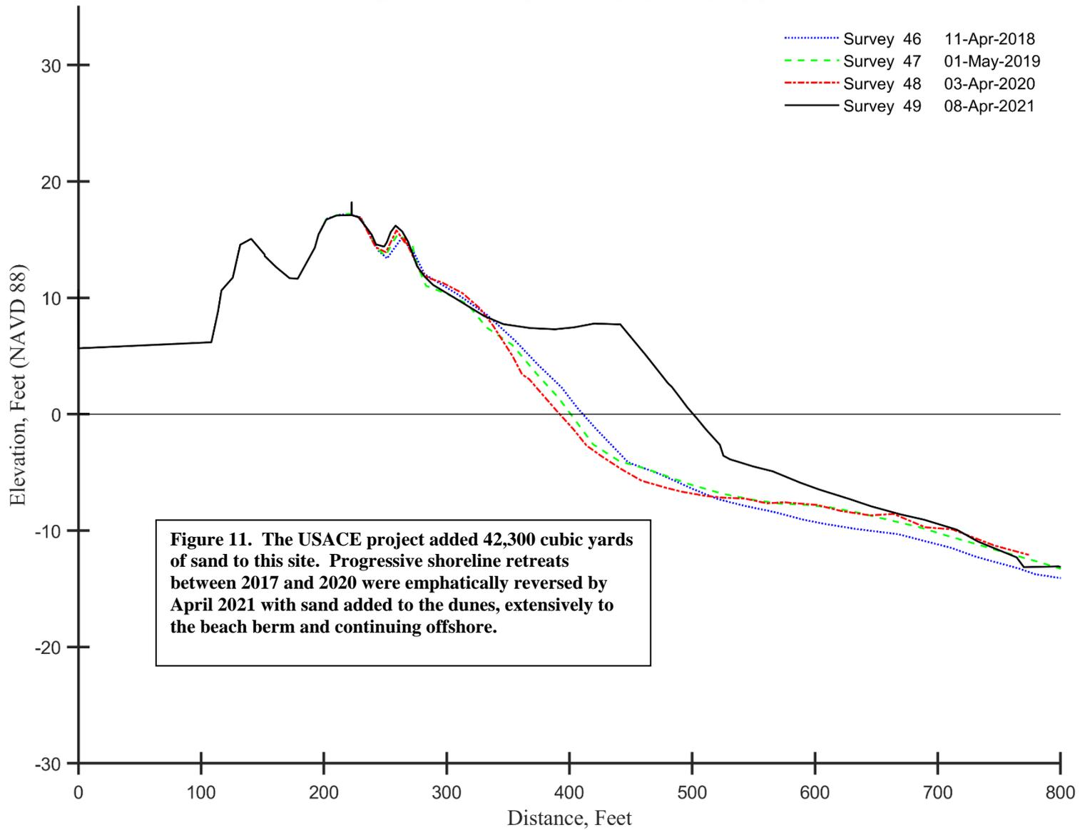
**Figure 11. The USACE project added 42,300 cubic yards of sand to this site. Progressive shoreline retreats between 2017 and 2020 were emphatically reversed by April 2021 with sand added to the dunes, extensively to the beach berm and continuing offshore.**
